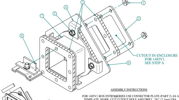
TEMPLATE. MARK, CUT CUTOUT HOLE AND DRILL .281" (7.1mm) DIA. HOLES. THIS IS TO BE DONE AT DESIRED POSITION IN ENCLOSURE.
