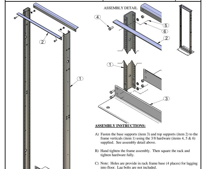
Note: holes are provided in rack frame base (4 places) for lagging into floor. Lag bolts are not included
