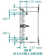
NOTE: - To maintain Type 12 & 4 rating, sealing washers must be used.
