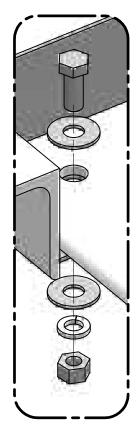
DETAIL A ASSEMBLY OF DOLLY TO RELAY RACK TYPICAL 4 PLACES
