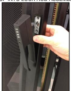
INSTALL 2 PROVIDED SCREWS (RETAINING BOLT NOT REQUIRED)
