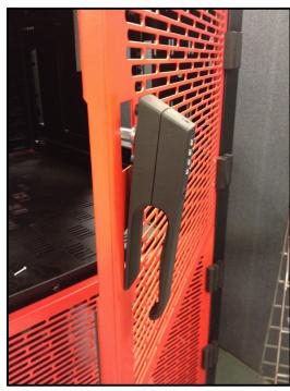
PLACE BOTTOM OF HANDLE IN CUTOUT FIRST THEN PUSH AND HOLD FLUSH WITH OUTSIDE OF DOOR
