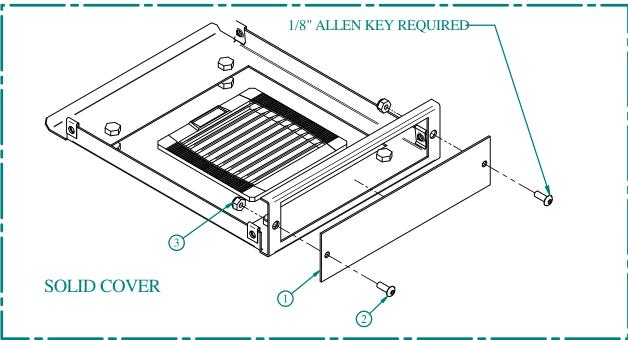
A) Fasten Grill/Solid Cover to the bottom of the rainhood using hardware provided.
