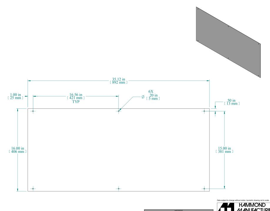
Material: 18 GA. (0.044") Cold rolled steel Mounting hardware included.
