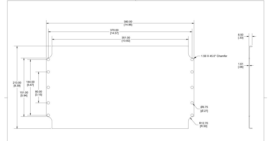
Enclosures can be Factory Modified (Milling, Drilling, Printing etc.) Contact Factory (modshop@hammfg.com) for quotes Solid models of this enclosure available in .stp or .x\_t (Part number and text placement/orientation on our products are subject to change, we do not recommend using them as a locating reference for modification purposes)
