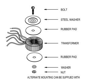
EPOXY FILLED CENTER HOLE FOR 5/16 BOLT
