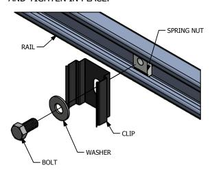
STEP 3 - WITH THE CLIP(S) INSTALLED ONTO THE RAIL(S) PRESS THE VERTICAL STRIP INTO THE CLIPS
