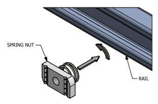
STEP 2 - ATTACHED THE CLIP WITH THE SUPPLIED BOLT AND WASHER TO SPRING NUT AND TIGHTEN IN PLACE.
