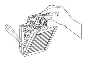
You can rinse the filter mat out using water heated to 40°C and commercially available mild detergent. It is possible to remove any dry dirt by knocking it out, vacuum cleaning it or blowing it out.
