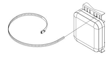
TO INSTALL BRACKETS ON POLE, START BY THREADING CLAMP THROUGH DESIRED SLOT
