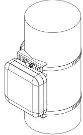
WHILE HOLDING ENCLOSURE AGAINST THE POLE, TIGHTEN CLAMPS WITH 5/16in (8mm) **NUT DRIVE**
