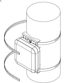
WRAP CLAMPS AROUND POLE AND THREAD THE CLAMPS **BACK THROUGH BRACKET**
