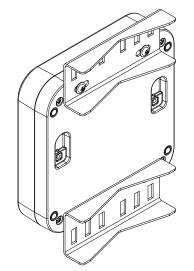
FOR #8 HARDWARE USE A #2 PHILLIPS HEAD. TORQUE ASSEMBLY TO 150 cN.m (13.5 lbf.in)
