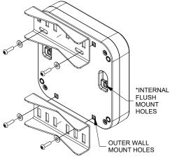
INSTALL BRACKET, WASHER AND SCREW TO THE OUTER WALL MOUNT HOLES.
